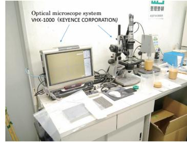
optical microscope for observation of the powders produced with L-8i
